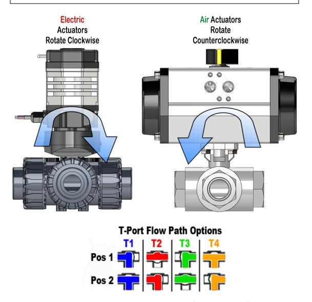
Actuated valves are assembled with either 4 bolts (METAL valves) or a 2-piece plastic kit (PVC valves). Remove the bolts that hold the valve onto an actuator to access the valve stem and rotate it to select the four possible 90° flow paths options from the columns marked T1, T2, T3 or T4.
