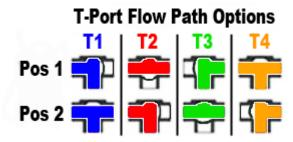
Moving the handle stop pin to one of the four outermost holes on the valve mounting pad allows selection of four possible flow path options (columns marked T1, T2, T3, or T4.) Each flow path option has two positions, as shown by **Pos 1** and **Pos 2**.
