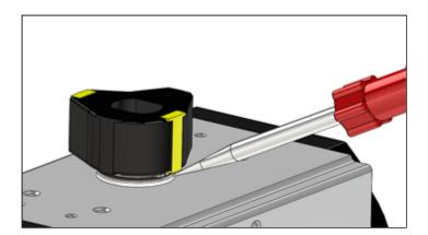
Yellow indicator tabs on air actuators may be changed to match the new flow path by prying each tab upward with a screwdriver as shown.
