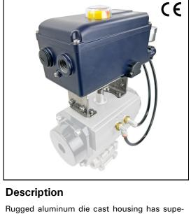
Rugged aluminum die cast housing has superior anti-corrosion surface treatment and an easy read visual valve position indicator. These positioners direct mount to rotary type air actuators with the standard VDI / VDE-3845 Namur style top shaft mounting. Universal Namur stainless steel mounting bracket kit is included with each positioner.
