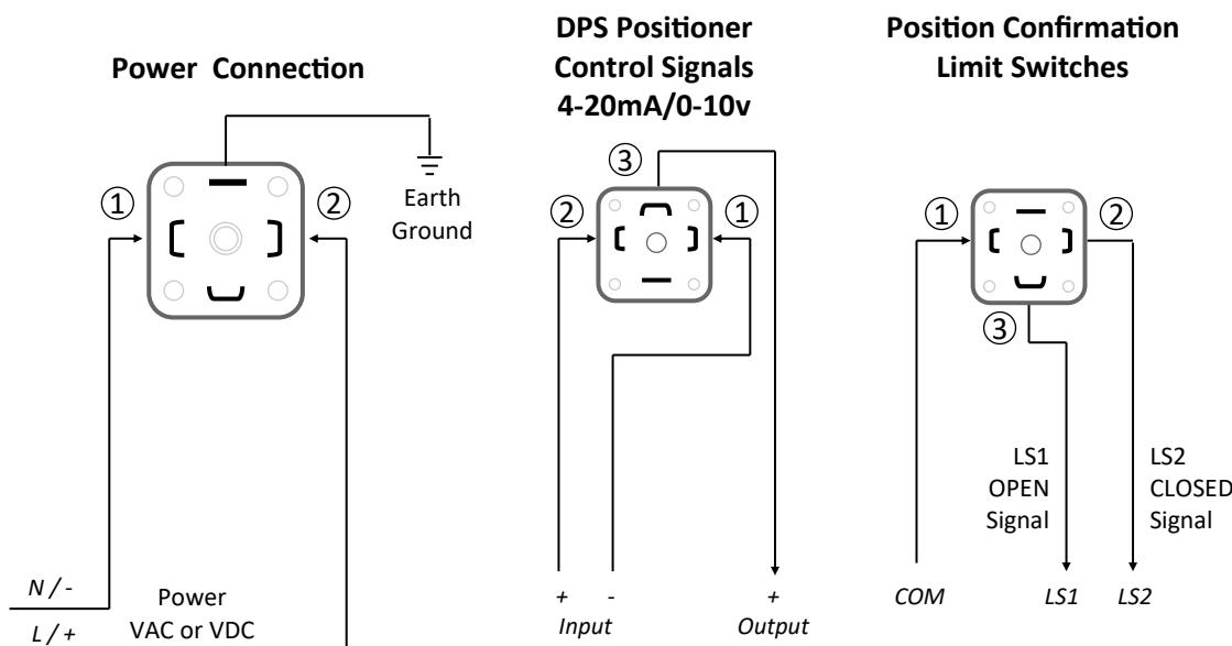
**Function: Actuators with DPS—Digital Positioner Option**
