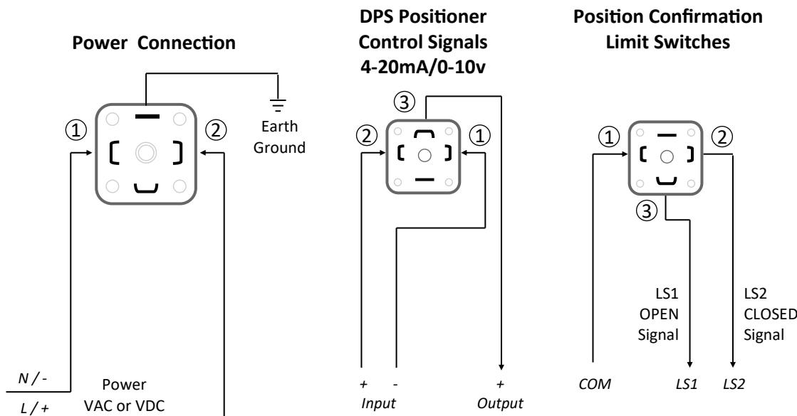
**Function: Actuators with DPS—Digital Positioner Option**
